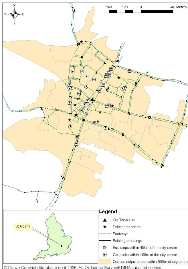
**Fig 2** The proposed layout of the new crossings, existing crossings with new dropped kerbs and the widened pavements
